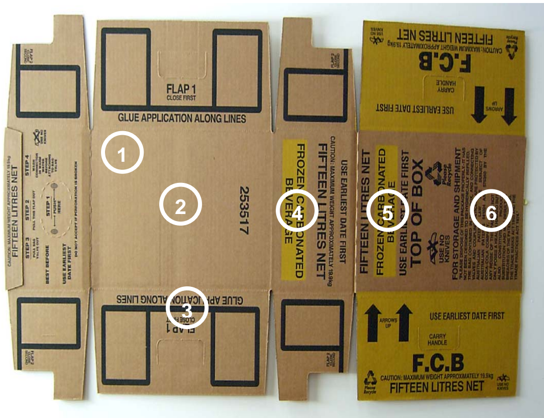
Figure 7. Example die cut box showing suitable sample measurements. Ensure that the same positions are measured on the way into the RDC to show conversion effects.
